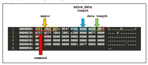
Figure 8. Initial packet sent by the client to the server (decoded)
