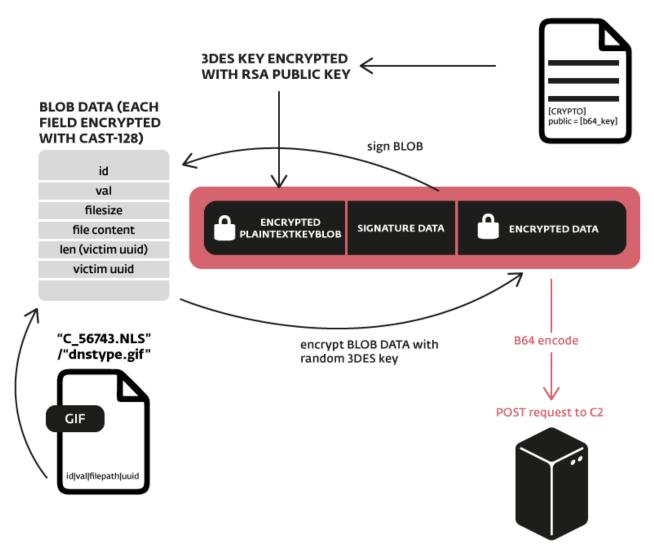
If the file "C\_56743.NLS" / "dsntype.gif" is not empty, it means there are data to be sent the C&C server. The file is parsed and the last line is retrieved. It contains details about the data to be sent. A data blob is built and each of the following fields is encrypted with CAST-128:
