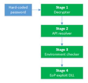
Figure 1. Execution stages of the exploit package and corresponding functionality
