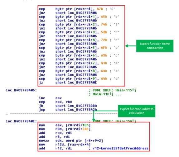
Figure 2. Locating kernel32!GetProcAddress location using EAT traverse
