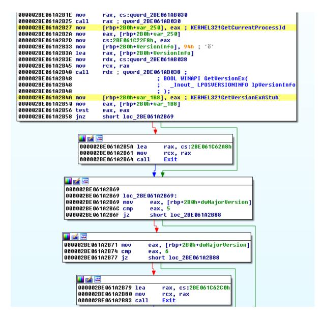
Figure 3. Code that performs environmental checks
