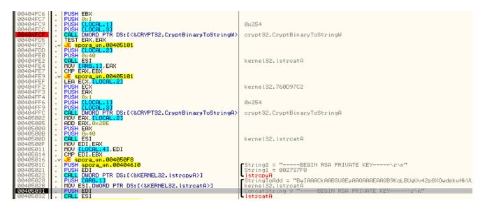
The formated version of the private key is stored in a buffer – along with the collected data about the machine and the infection, including: date, username, country code, malware sample id, and statistics of encrypted file types.
