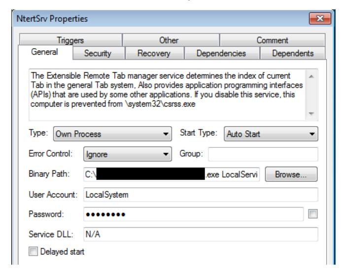
Figure 1 Disttrack service created on systems during propagation
