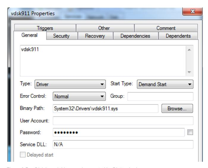
Figure 2 RawDisk kernel driver service created by Disttrack wiper
