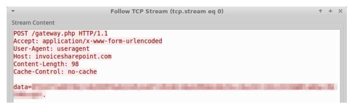
Figure 5: ScanPOS exfiltrating CC data over HTTP
