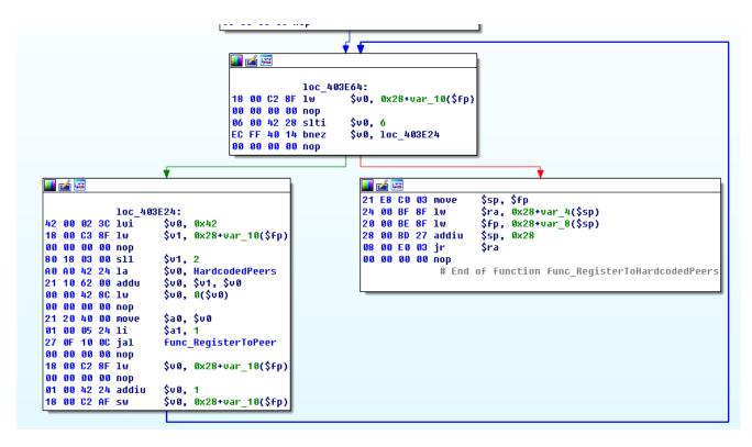
Figure 7 register to hard-coded peers
