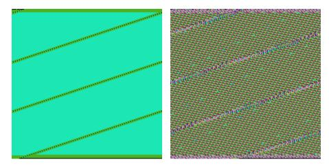
Indeed, again we can see patterns of original content reflected in the encrypted content, that suggest that some block cipher has been used. We can suspect, that also in this case it is AES in ECB mode.
