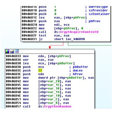
Just like it was before, a file is read and divided into chunks. Then, the random key along with the buffer containing a single chunk is passed as a parameter to a new encrypting thread. For the content encryption, the same AES implementation like in the previous versions has been used.
