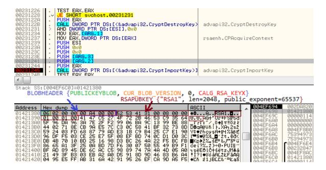
The RSA key is used to encrypt AES keys, which are randomly generated for each file.
