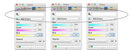
Figure 7. Effect of flipping one and two bits from each color channel. The circle around the three white rectangular regions shows how the white color changes slightly as the number of bits is flipped. (Source: Dell SecureWorks)
