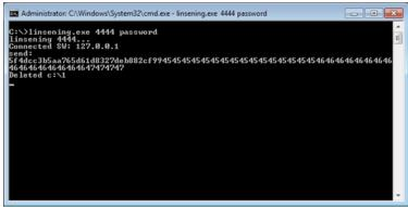
Figure 1. LinseningSvr sending hashed password and 36 bytes of data. (Source: Dell SecureWorks)
