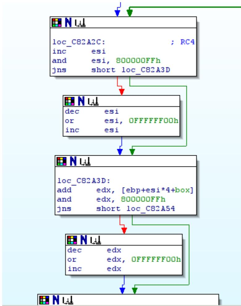
So the config file is crypted with RC4 with the key “CONFIG”.
