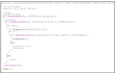
Figure 3. The function in ZeuS which reads data from the registry
