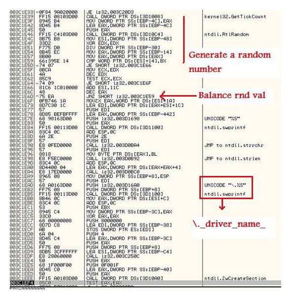
We have an interesting algorithm here, after driver enumeration a random number is generated, next fitted within a range of [0 - 0xFF] and used to randomly select from the driver list a file to be infected. Finally the string formatted as:
