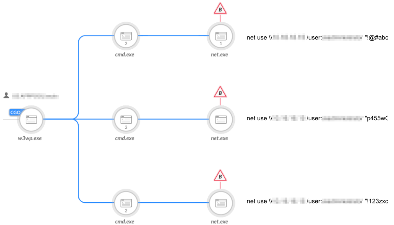
Figure 7. Password brute forcing using SMB.
