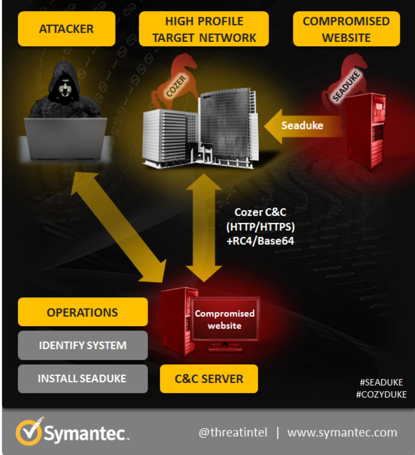
Figure 2. How the attacker tasks Cozer to install Seaduke
