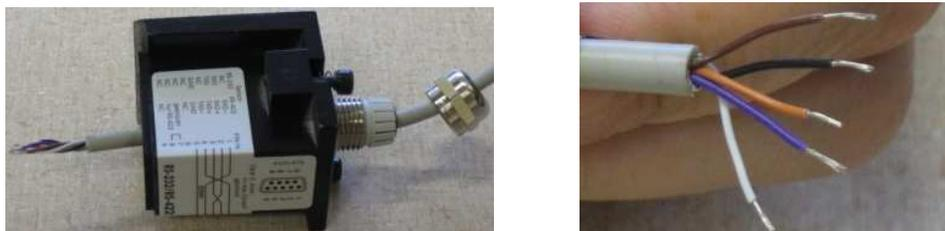
Figure 5: (Left) After properly mapping the inner wires to their respective pins, thread the data cable through the cap and then through the block. (Right) Wires lined up according to the mapping after being threaded, pin 5’s wire is white, pin 1’s wire is brown.
