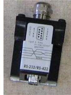
Figure 1: (Left) The USB-COMi-M USB to RS-232/422/485 Industrial Adapter can be used to enable the fastest Sick LMS 2xx data rate of 75Hz. It is a popular alternative (in both industry and academia) to the proprietary Sick adapters, which are nearly an order of magnitude more expensive. (Right) The Sick LMS 2xx Data Terminal Block w/ DB-9 Male Connector.
