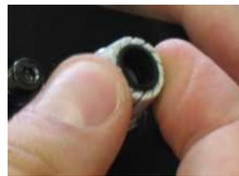
Figure 2: (Left) Remove the gray cylinder from the Sick cable block. (Center) Remove the plug by poking it out with a screw driver. (Right) Reinsert the cylinder back into the Sick data cable block.
