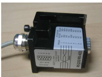
Figure 8: The final assembled data block terminal for the Sick LMS 2xx.
