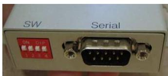
Figure 9: USB-COMi-M jumper configuration for RS-422 communication.
