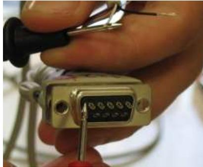
Figure 4: Identifying the white wire using the connectivity setting of the multimeter. In this case, a loose male DB-9 adapter was affixed to the female end of the altered cable making it easier to probe and measure the outputs. To measure connectivity (in this case for the the white wire), we hold a single probe (the black probe) to the exposed part of the wire and then test each of the pins on the other end (with the red probe) until the multimeter indicates connectivity.
